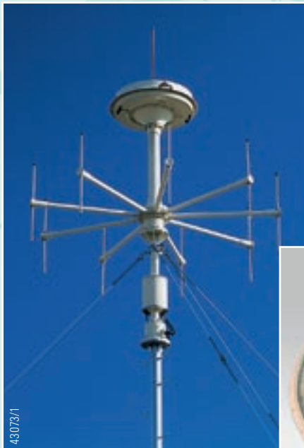
FIG 4 DF antenna system for 20 MHz to 3000 MHz in stationary use.
