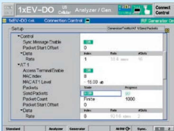
FIG 3 Comprehensive configuration capabilities for access network simulation.
