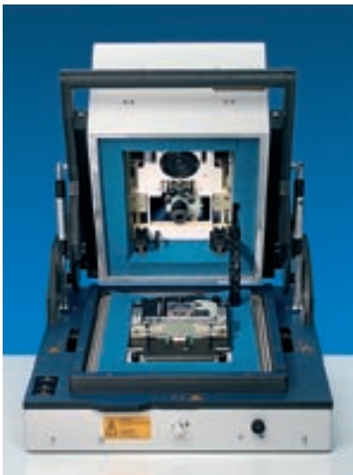
The new Shielded RF Test Fixture R&S®TS 7110 can accommodate completely different tests, from initial board tests to complex final tests (function tests) of mobile phones and other small equipment (page 4).
