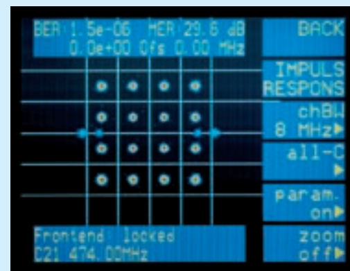
FIG 4 Constellation diagram of an OFDM signal.
