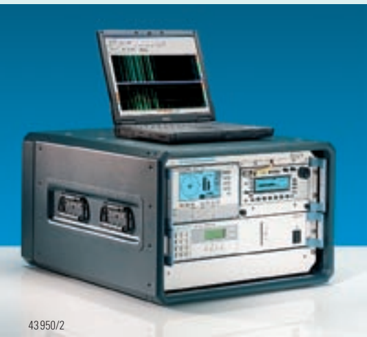
FIG 3 The R&S®TMSR with a detachable R&S EB200 receiver for manpack operation.
