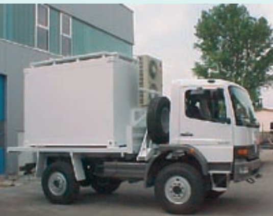
FIG 4 Semi-mobile radiomonitoring and direction-finding station – ready for transport.
