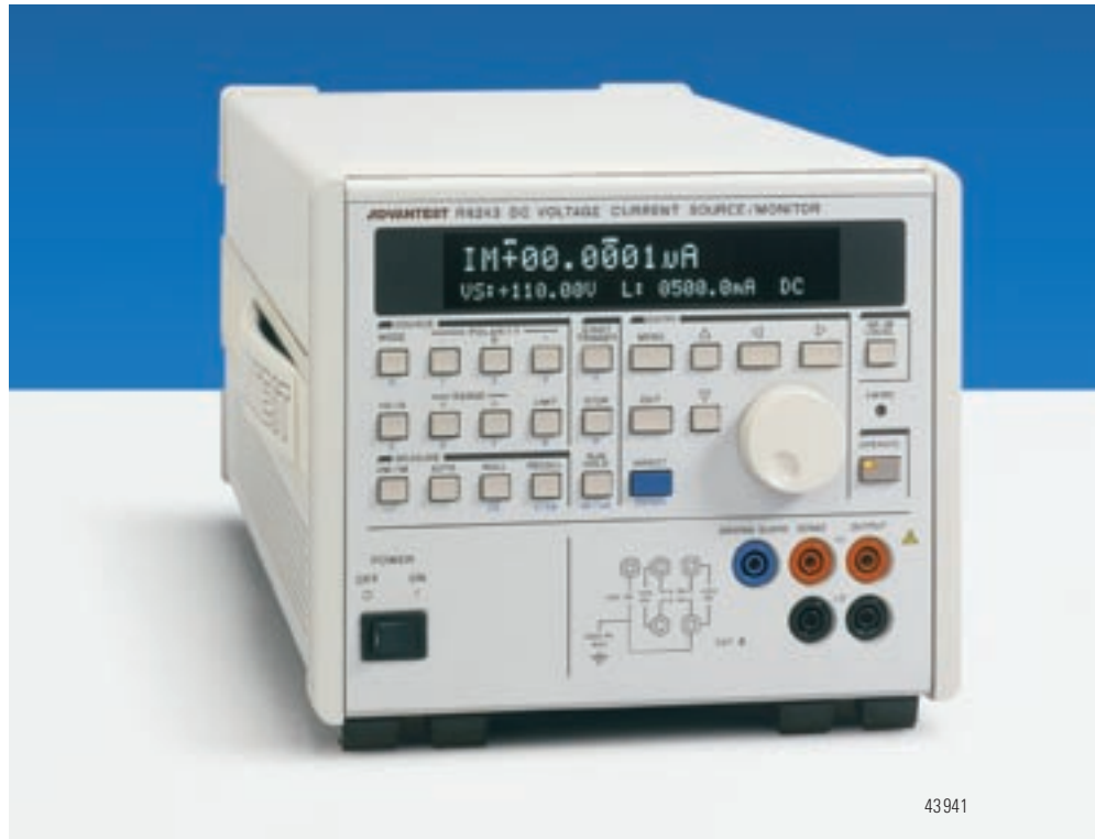
FIG 1 The bipolar DC Voltage Current Source/Monitor R6243 is equipped with a guarding connector (blue) which, during operation in the lower nA range, compensates for measurement errors caused by parasitic external capacitance.
