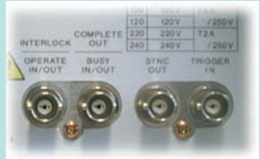
FIG 7 Versatile: The BNC female connectors on the voltage/current sources sometimes feature multiple assignments and are preset with different functions.
